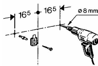
Fastening on the wall, reglage from 33 to 17 cm
